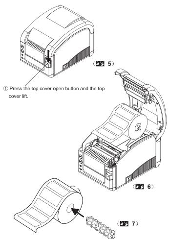
② Insert the paper roll spindle into the paper roll, and adjust the spindle position to make it in the center of the paper roll.
